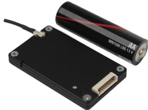
The transmitter can be pre-set to 3 separate frequencies (within 1MHz) anywhere in the band 300MHz to 1GHz, making it suitable for most applications.
